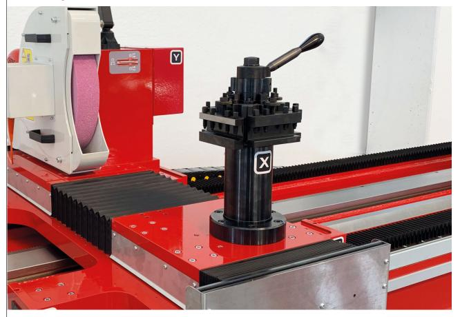
Designed to equip the Prima Grinder with up to 4 tools for the different cutting, facing or re-work of the grinding wheel.
