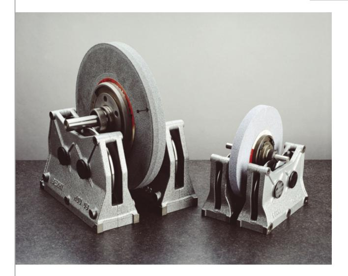
Instrument needed for a correct manual balancing of the grinding wheels; this is a frequent and needed activity for a proper execution of the grinding process. A solid design connected to a specific selection of special bearings suitable for this application generate the ideal conditions for the balancing operation. A special shaft with a grinding wheels flange for the Prima Grinder are included with the supply.
