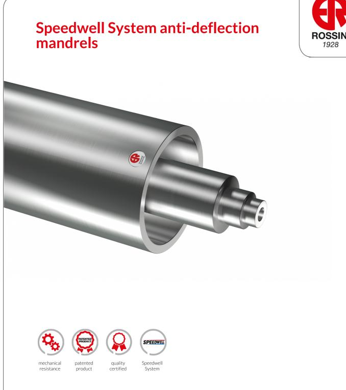
Special anti-deflection design of the mandrel for using the rubber Speedwell sleeves in heavy-duty applications. The mandrel has the patented tapered value, a close chamber distribution system for the compressed air and moreover the perfect grinding of the surface that can be supplied with chrome, nickel coating according to the manufacturing drawing for the easy and proper mounting of the rubber Speedwell Sleeves.
