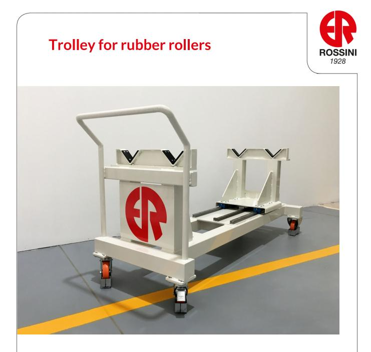
Mainly designed as ancillary for the PRIMA GRINDER. It allows the handling of two rollers (i.e. one for loading and one in download from the machine to the storage or usage point) in a dimension range from 1100 to 1700 [mm] variable distance between the supports, a diameter up to 300 [mm] and a maximum weight of 400 [kg]. The trolley can be used also to carry mandrels, shafts, sleeves or anilox. It can be designed according customer's request.
